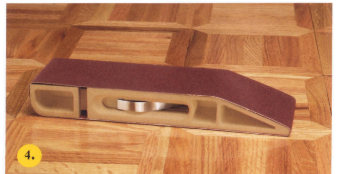
4. The belt is now securely locked and loaded and ready for extended sanding action.
