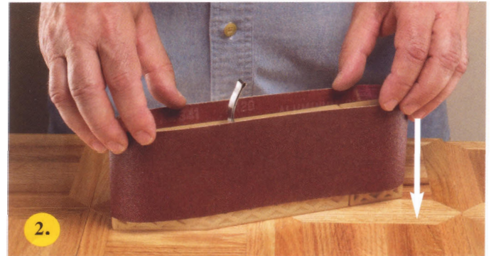
2. With the lever still open, slip the new belt on the SandDevil.
