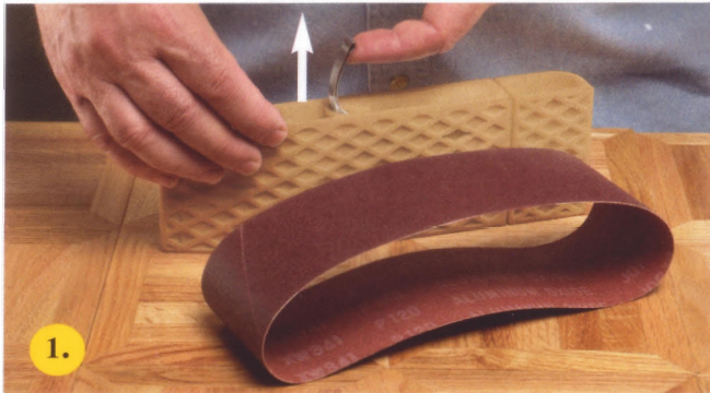
1. Lift the lever up to contract the SandDevil. The belt is now easily removed.
