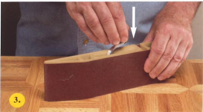
3. A light downward push on the lever expands the SandDevil and keeps the belt securely in place.
